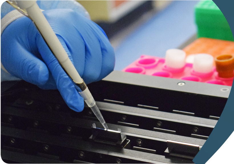
Microarray technologist Sarah Miller (above and on the cover) adds staining reagents to the array that enable fluorescent detection of methylated and unmethylated areas of the DNA.
